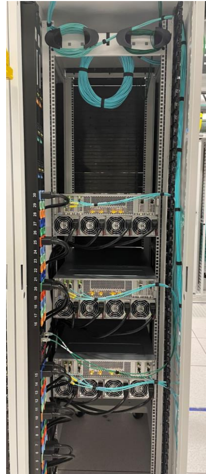
SuperMicro Server c/4xGPUs NDR 200G Transceivers a 850nm
