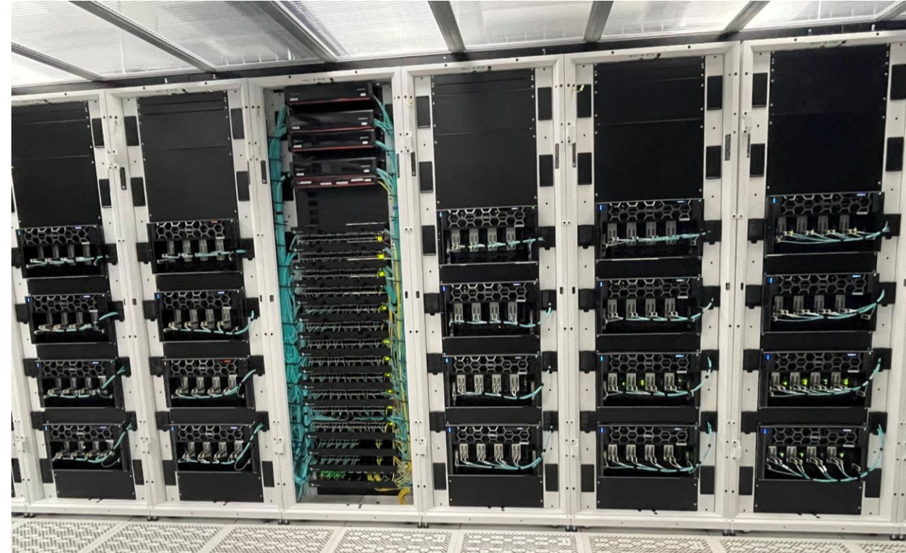
1 POD or Scalable Unit with 5 server cabs + 1 network cab
